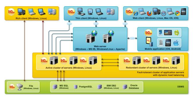
1C:Enterprise uses industrial DBMS (Oracle Database, IBM DB2, MS SQL Server, or PostgreSQL), which allows building high-performance and reliable information systems. The thin client and the web client support user work over the Internet, including mobile communication channels. The web client does not require pre-installation on a user's computer.
